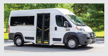
Chassis: Ram Promaster 2500, 159" High Roof Window Van Engine: 3.6L PentastarTM Variable Valve Timing (VVT) V6
